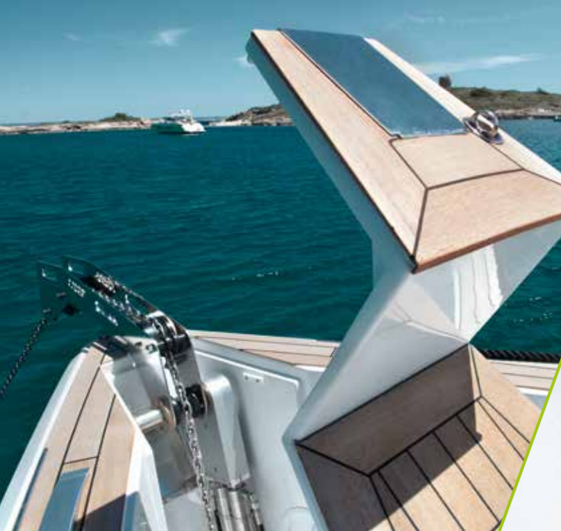
easy to use: the hydraulic anchor launching system
