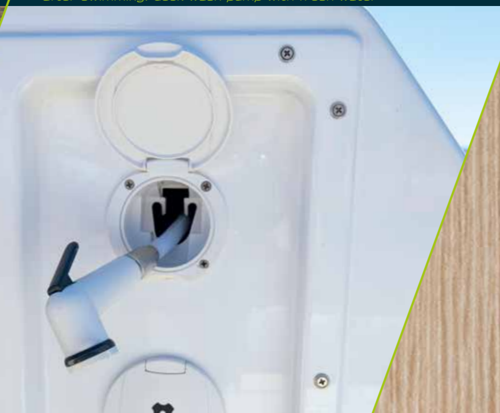
after swimming: deck wash pump with fresh water
